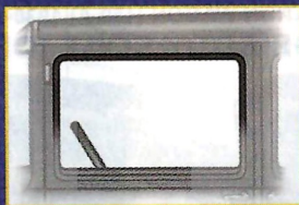
Briggs: straight top of door window opening
